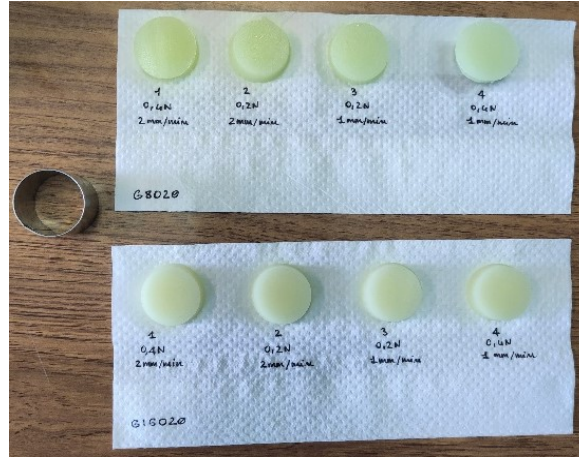
Figure 2. 4: Samples derived from the G8O20 (top) and G16O20 (bottom) phantoms, numbered to indicate the different mechanical measurement conditions under which they were tested. For both the G8O20 and G16O20 sample ‘1’ was measured with 0.4 N preload and 2 mm/min test speed (PL04TS2); sample ‘2’ was measured with 0.2 N preload and 2 mm/min test speed (PL02TS2); sample ‘3’ was measured with 0.2 N preload and 1 mm/min test speed (PL02TS1); sample ‘4’ was measured with 0.4 N preload and 1 mm/min test speed (PL04TS1).
